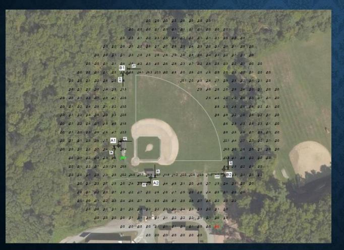
With specially designed field lighting, light focus on playing field only with no additional light pollution for surrounding area
